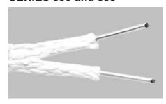
The SERIES 350 uses the ultimate high-temperature flexible insulating system. The ceramic fiber yarn's upper temperature limit often exceeds the melting point of the material it's insulating. When an application requires flexible insulation, while pushing Type K or Type N to their extreme limits, ceramic fiber insulation is the only choice.
