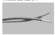
SERIES 511 is the most economical polyimide taped construction. The polyimide film applied to the conductors is considered to be the ultimate "soft" insulation. The tape maintains its strength at temperatures to 315°C (600°F). The FEP laminate serves as a moisture barrier and allows the tape to fused with itself. The finished construction will not unravel when cut.
