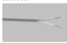
The SERIES 506 is the smallest standard insulated wire construction. The thin FEP wall on both primary and duplex insulation yields a construction that can operate safely at temperatures far beyond common PVC and nylon insulations.
