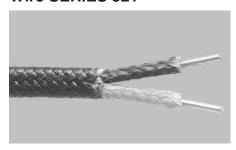
The addition of color coding and impregnation to the high temperature fiberglass make this the logical next step for systems which have exceeded the temperature capabilities of standard glass insulated series.
